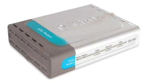
Modems can be external, connected to the computers serial port by an RS-232 cable or internal in one of the computers expansion slots. Modems connect to the phone line using standard telephone RJ-11 connectors.
