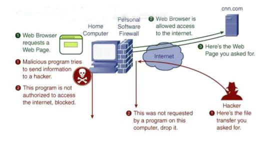
A firewall has the basic task of controlling traffic between different zones of trust. Typical zones of trust include the Internet (a zone with no trust) and an internal network (a zone with high trust). The ultimate goal is to provide controlled connectivity between zones of differing trust levels through the enforcement of a security policy and connectivity model based on the least privilege principle.
